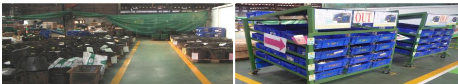
Fig.1 The area of the furnace section before (left) and after (right) the application of worksite control with 2S resulted in the introduction of Flow Rack to facilitate FIFO system.
