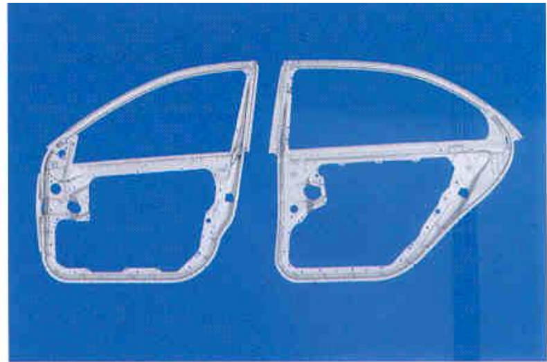
Fig. 2. Door inner-frame using aluminium pressure diecasting (picture GF Automotive)
